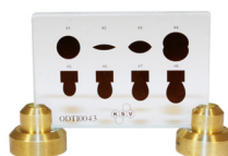
Contact angle and surface tension calibration kit ref. C216A
