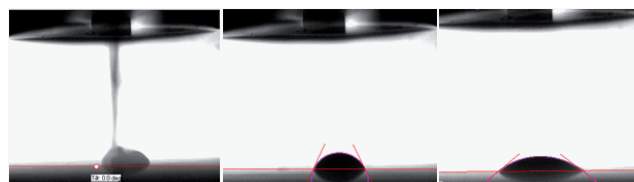
Figure 3. High speed camera enables to measure the initial picoliter drop contact angle right after the drop hits the surface and then the fast spreading and absorption phenomena.
